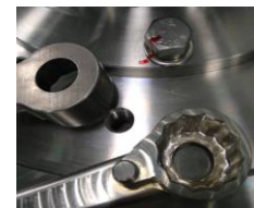
⑦ 固定螺栓每颗螺母都有 标线作记号 ⑦ Fixing bolts (for each nut) Marking
